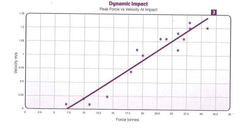
designed measurement system capable of fast sampling. Correlation between peak impact force and peak acceleration has been established and showed linear relationship within reasonable confidence limits and allowed an estimate of the vessels added mass. Correlation between impact force and initial impact velocity also correlated well with a linear relationship.
